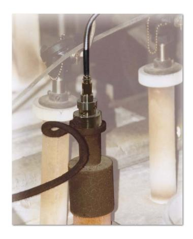
The pyrometer IS 50-LO/GL is specially designed for the glass industry. It is used for the temperature measurement of glass in tank, working end, forehearth and feeder. Additional applications are the measurement of brickworks in regenerator and tank.
