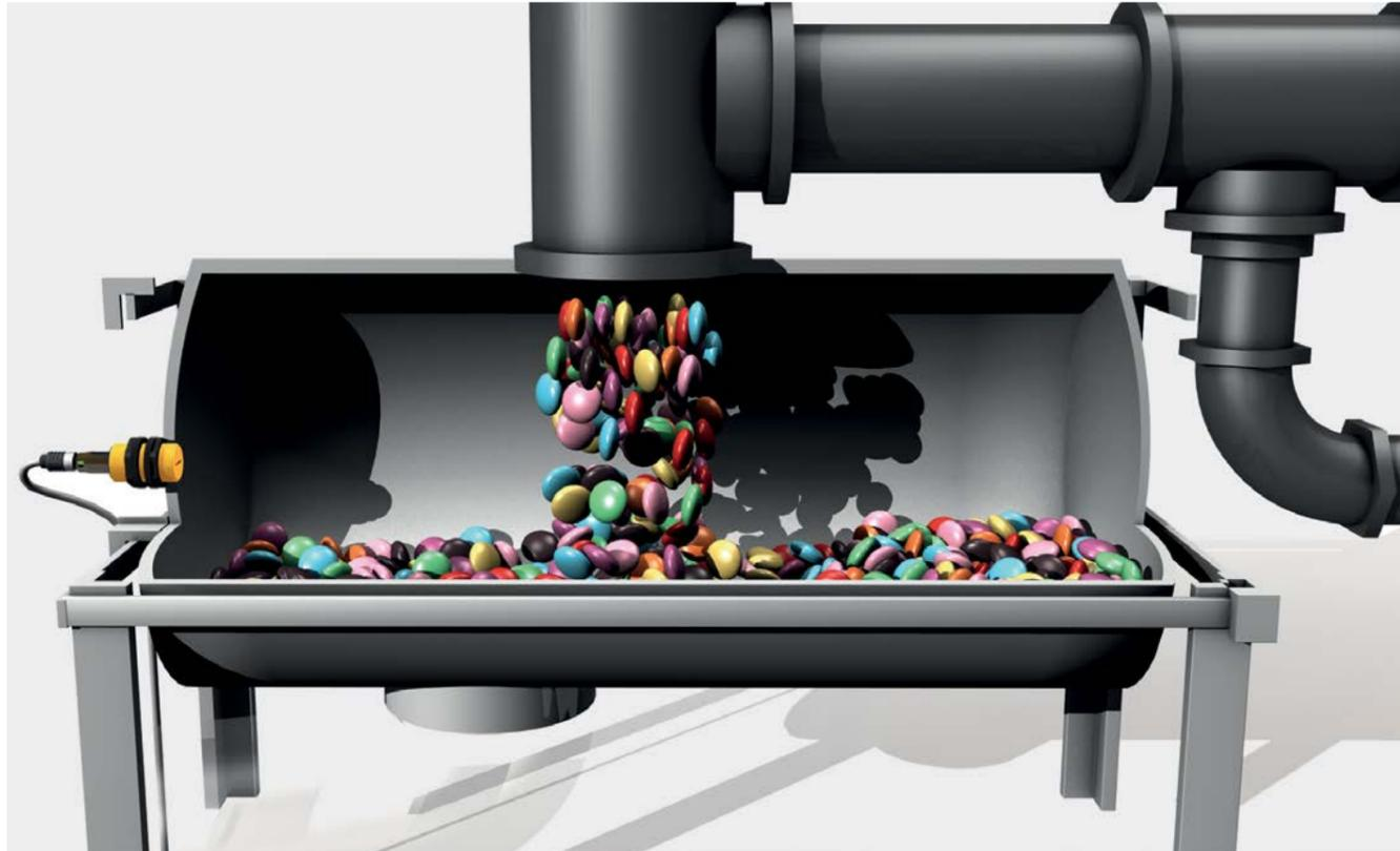
In industrial automation, capacitive sensors are used to detect a variety of media and are most frequently used for monitoring the fill levels of liquids or bulk goods. In the plastics, packaging, and chemical industries, as well as in mobile work machines – Turck's BCT sensors reliably detect all solids, liquids, metals, and non-metals,
