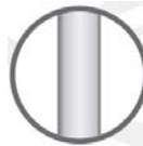
Typical 1.5" gas wafer flow meter. Bluff body blocks 43% of pipe cross-sectional area.
