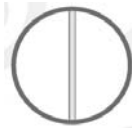
Racine Vortex 1.5" gas wafer flow meter. Bluff body blocks 9% of pipe cross-sectional area.
