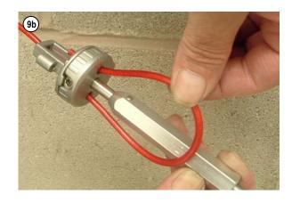
10a. The rope is then pulled by hand through the Tensioner / Gripper to take up any slack rope before final locking.
