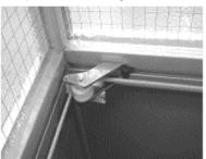
4a. For 2 switch systems, up to 50m., undo the locking clasp on the Quick Link (QL) locking and fit the clasp fully around one of the switch eyebolts.
