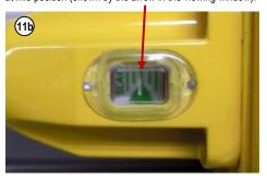
11c. For long rope spans >50m. it is advisable to balance the system by making turns to the Left and Right Tensioner/Grippers in turn whilst at the same time checking the rope tension setting in each of the switch viewing windows.
